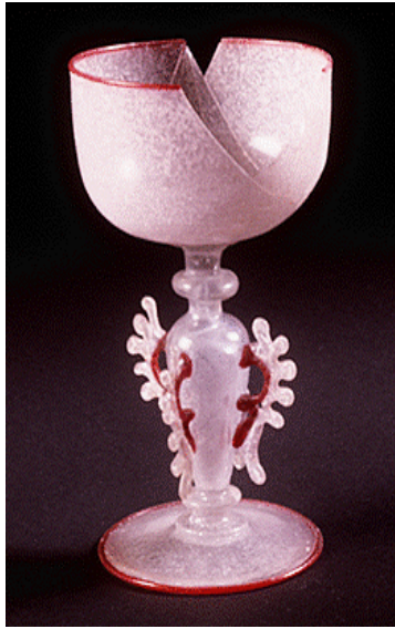
Figure 2. An example of Vessel glass decay in an 18C Venetian goblet. The glass is too rich in soda rendering it unstable to moisture. The frosty appearance is the result of crizzling which has led to mechanical failure.
