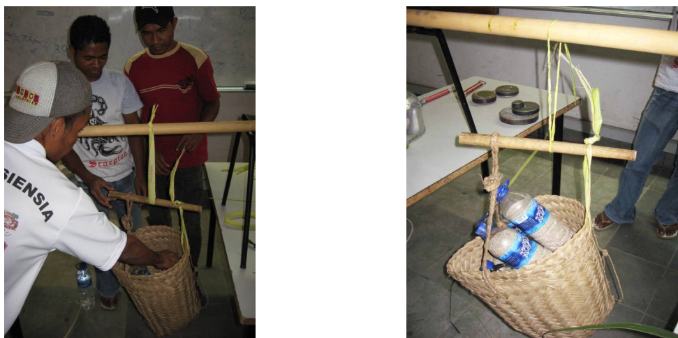
Figure 4. Students are testing tensile strength on leaves from different species of palm and of different ages. Weight is added to the basket until breakage occurs, and then the weights at which catastrophic failure are added up. Results are then graphed and compared with the students' predictions.
